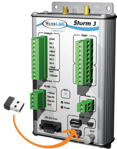
Figure 7: Insert Wi-Fi adaptor
