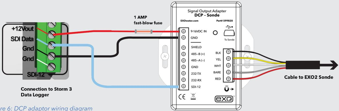
Figure 6: DCP adaptor wiring diagram
